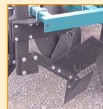
Shear bolt safety feature on all furrow shanks
