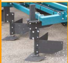
Furrow shanks with wings lead the shaper pan to dig furrows. Furrow shanks feature replaceable sweeps.
