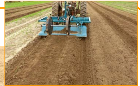
Finishing Bed Shaper equipped for light tillage
