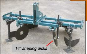
Furrow shanks and shaping disks are standard equipment and rugged for small farm service. Buckeye Bed Shapers pull straight with less HP.
