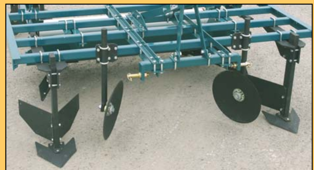
Furrow shanks and shaping disks are standard to fill bed, pull straight and pull with less power
