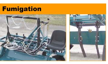
Fumigation knives and tank rack are available for Model 4612. Compatible with tape applicators and other options.
