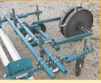
Puncher wheels trailing a Mulch Layer are very practical to get ready to plant.
