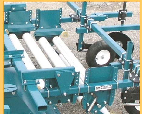
Equip with double roll carriage for non-stop operation on long rows
