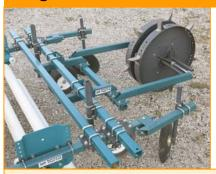
Puncher wheels trailing a Mulch Layer are very practical to punch through plastic and mark plant locations at the same time.
