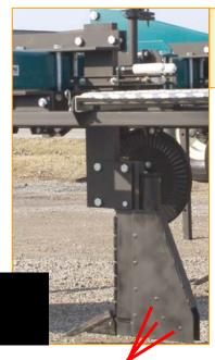
Connectors turn on THREE rollers, arrayed on 10" circle
