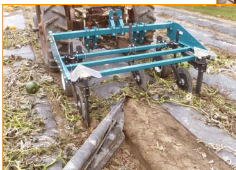
The strategy for plastic mulch is to split it down the middle then pull or wind-up each half by hand or by machine
