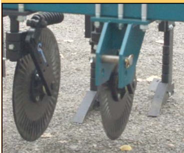
TYPICAL SHANK SET-UP FOR DRIP TAPE
