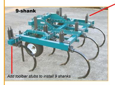
Rugged 1-piece frame for tractors up to 135 PTO-HP
