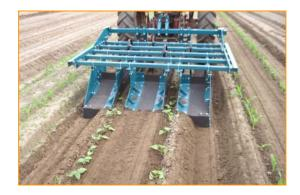
Rolling soil action in front of shaper pan buries starting weeds.
