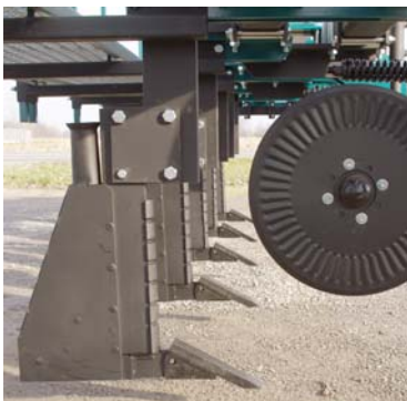
50 HP Shank for application below plow level
