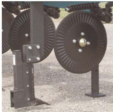
25 HP Shank for application below seedbed
