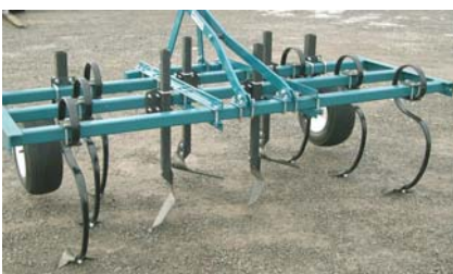
Row crop cultivator with S-tines and beet sweeps. Many attachments available to master mechanical weed control
