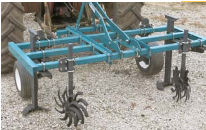
Re-configure mulch lifter and add sweeps and row spiders to cultivate between mulch rows
