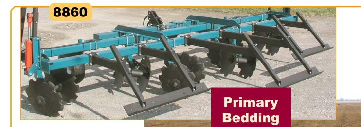
3-bed Disk Bedders quickly rough-in beds over big acres to allow beds to settle before bed finishing. Soil can be wet or cloddy after post-harvest primary tillage. Notched disk blades cut through residue and bedding action further mixes or buries residue. Use GPS or add row markers for accurate bed spacing.
