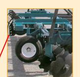
Gauge wheels for depth control are standard equipment.
