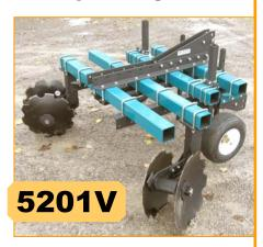
Disk gangs are set-up on 5201V to throw soil toward vines. This features the same hitch as 5201 and is available with different toolbar widths to match your row system or a 4th toolbar (shown) for adjustable frame width. Attachments are available to loosen harder ground or heavier sod in front of gangs - please inquire. Ask about hydraulic on-the-go width adjustment.
