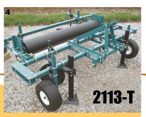
Row tunnel application may involve working in tractor wheel tracks. Model 2313-T features a heavier hitch and front tillage shanks to loosen wheel track compaction ahead of opening disks. These features can be retro-fitted to 2113.
