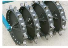
Many wheel choices available for close plant spacing, starting at 4". Garlic spacing is typically 6". Removable punches allow wheels to be used for other crops.
