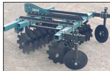
Bed Harrows cut up heavier residue and keep beds intact
