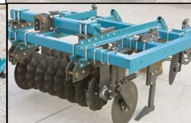
5500 Bed Reconditioners are all-in-one machines for moderate to heavy residue
