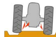
Wheel spacing too narrow or bed tops too wide present several problems
