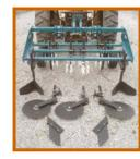
2" square toolbar frames can be equipped with an open-center hitch for accurate placement of parts with several set-up - no conflict with hitch parts
