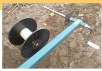
Storage spools save tape for reuse or move grids of drip lines during irrigation season. Spool can then be mounted on drip tape applicator
