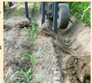
A basic illustration of beet knives placed close to the row and crescent hoes cultivating raised bed sides
